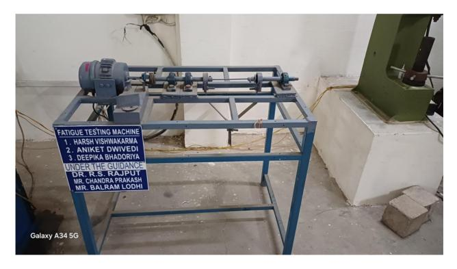
The in- house facilities of workshop and fabrication shop have been utilized for the same. This machine is used to test endurance strength of materials under cyclic loading conditions.
